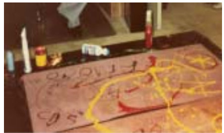
Sample carpet with mustard, ketchup, shoe polish, hair dye etc. smeared on it
