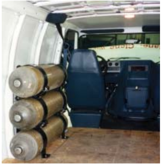
Tanks may be mounted inside or outside the vehicle.
